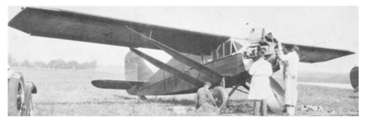
Bellanca #14. The ring cowling for the J6-9, seen lying on ground, was poorly installed and caused delays during the tour. Note mechanic using bucket for work stand.
