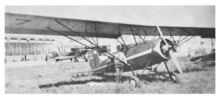
Harvey Mummert and Mercury Chic. The Chic had an unusually high parasol wing, which made it difficult to handle on the ground, and full span ailerons, actuated by push-rods which slanted out through cockpit coaming.
