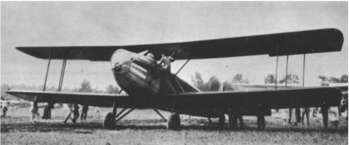
The Douglas C-1, Pathfinder and Official Press plane. Pilot and mechanic sat in cockpit just behind. Liberty motor; eight passengers rode in enclosed cabin. (Ford/Hudek)
