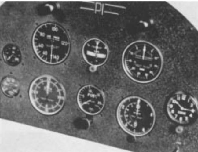
Pioneer Travel Air had conventional round dial instruments in front, vertical scale in rear cockpit. Blind flying instruments included Air Speed, Turn and Bank, Pitch Attitude, Earth Inductor Compass, Rate of Climb, and Air Log.
